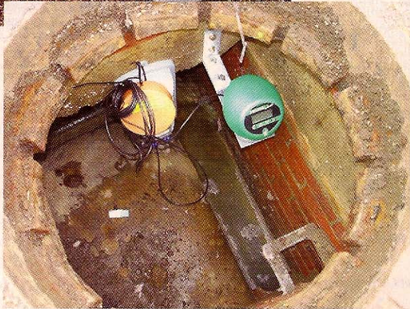
Figure 1. Collecting network information effectively in real time requires devices that can operate at low-power and with wireless communications.
